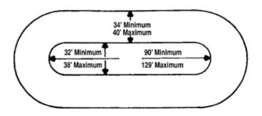
Diagram 3-2 Speed-breaker Detail
