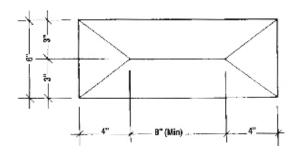
Diagram 3-3 Speed-breaker Elevation
